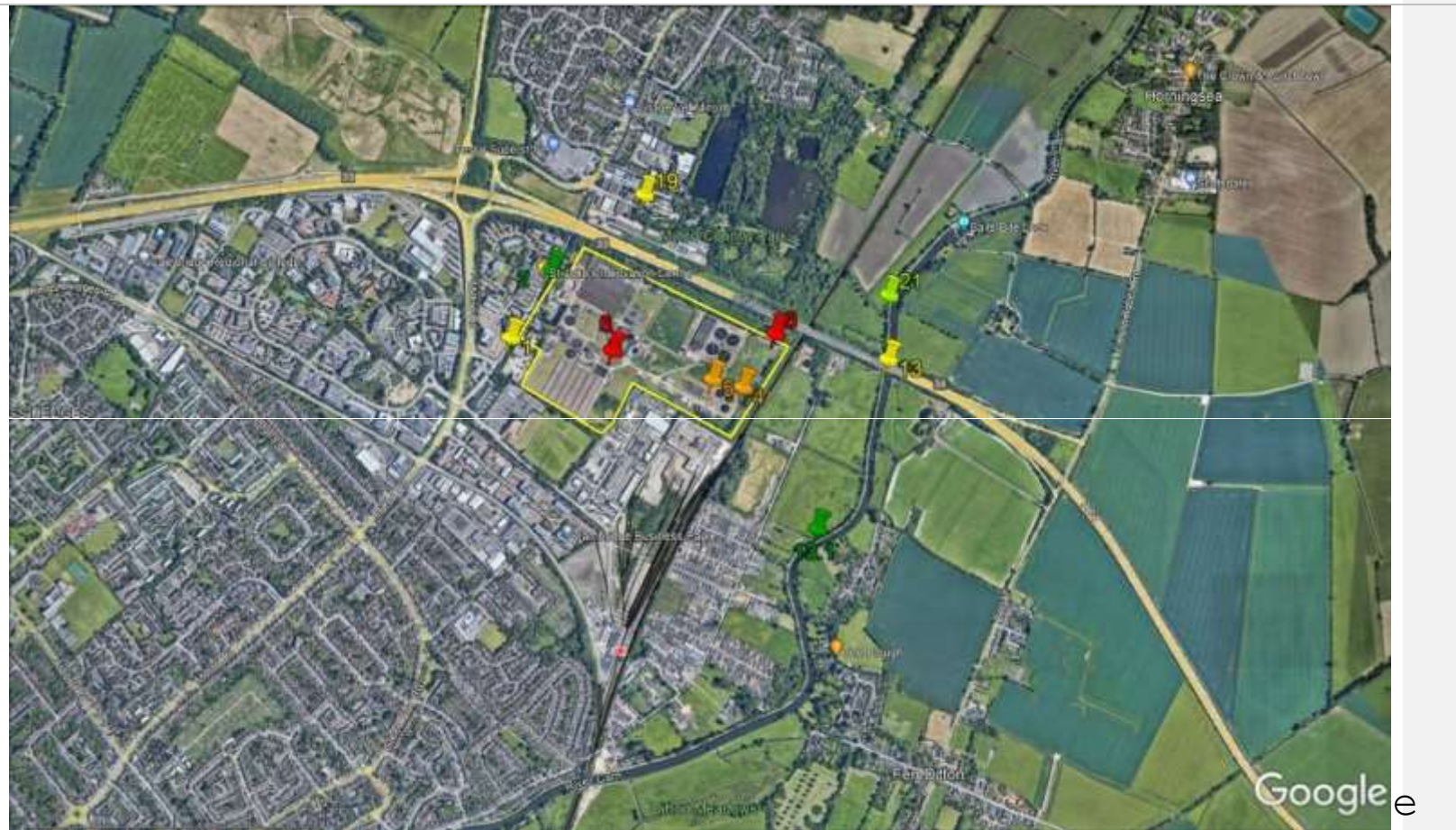
Figure 11: Sniff Survey 2 – Colour coded pins based on highest Odour Intensity Mean results for locations where 'relevant' odour(s) were detected
